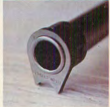
Above: Special bushing is fitted to all guns and handfitted to barrel for maximum rigidity when gun is in battery. This allows each shot to go into same place due to identical barrel, slide, frame relationship.
